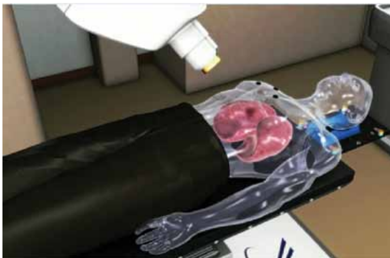
The Synchrony System is capable of tracking a wide variety of target motions, including targets that move with respiration. Changes in breathing pattern are automatically detected by the Synchrony System and compensated for in treatment delivery.
